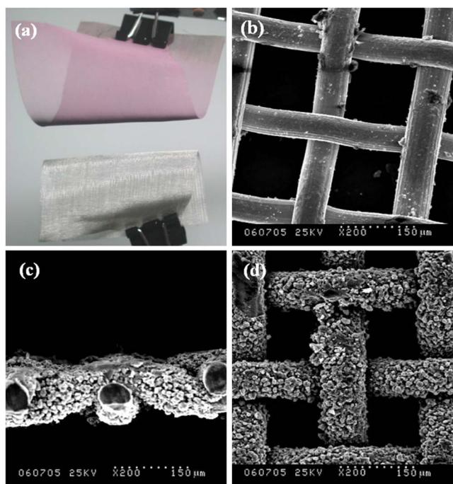
FIG. 1. (Color online) (a) Optical photo of the as-prepared electrode (upper,  $4.5 \times 7 \text{ cm}^2$ ) and the net substrate (lower,  $4 \times 5.5 \text{ cm}^2$ ); (b) SEM photos of the mesh substrate; [(c) and (d)] top and sectional views of the as-prepared electrode.
